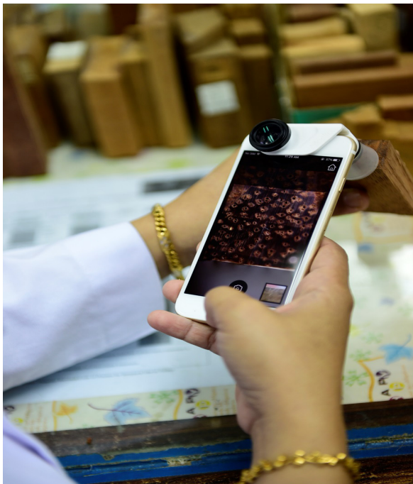
3. Place the Iphone 6/6s/7 with olloclip macro-lense (21×) on the surface prepared earlier, and click 'capture' in the application
