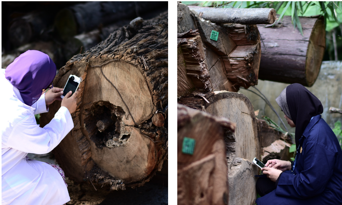
Figure 2 Timber group identification of logs using the MyWood-ID application
