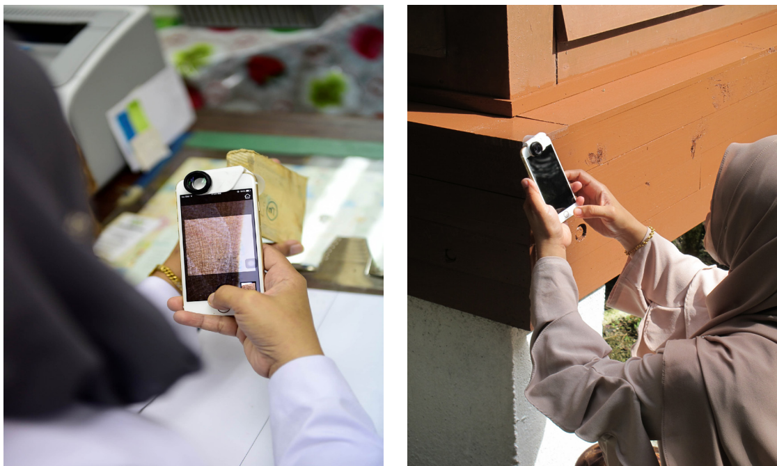
Figure 3 Timber group identification for building and small wood sample using MyWood-ID application
