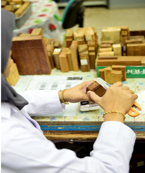
1. Prepare a clear cross section using a sharp cutter
