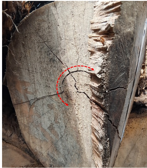
Figure 3 Ring shake in a Fagraea fragrans
