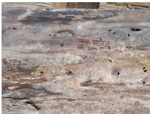
Figure 5 Small holes in Tectona grandis caused by wood-boring insects
