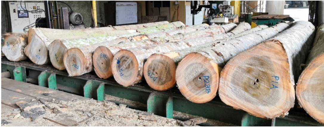
Figure 9 Logs of Paulownia with a rounded-hollow pith
