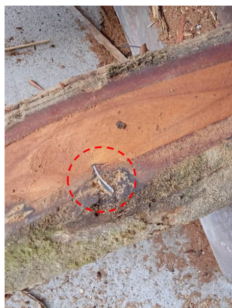
Figure 17 An embedded metal plate in Terminalia sp. log
