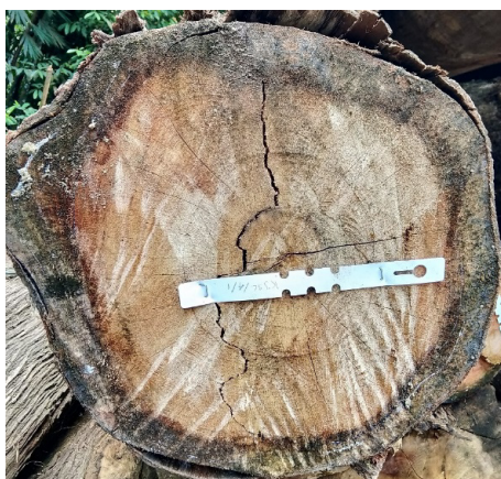
Figure 14 Internal non-linear cracks due to felling impact
