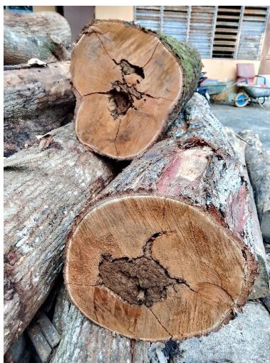
Figure 7 Hollow logs of Acacia hybrid filled with termite nest
