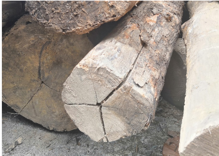
Figure 1 End checks and splits in Tectona grandis
