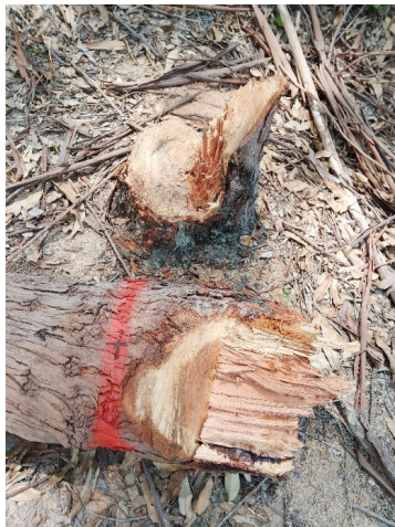
Figure 11 Splintering fracture of Eucalyptus hybrid log due to improper felling cut
