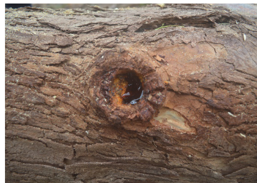
Figure 6 Medium hole of decayed knot in Eucalyptus hybrid
